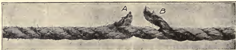
Fig. 1. A Broken Strand to Be Repaired.
